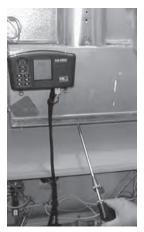
While a carbon monoxide analyzer is a good instrument for CO safety, a high quality combustion analyzer can be used for safety checks, combustion diagnostics and precision burner adjustments. Residential/light commercial combustion analyzers range from \$600 to \$1,500, depending on quality and accessories. Some of the important features to look for in a combustion analyzer are fast response
